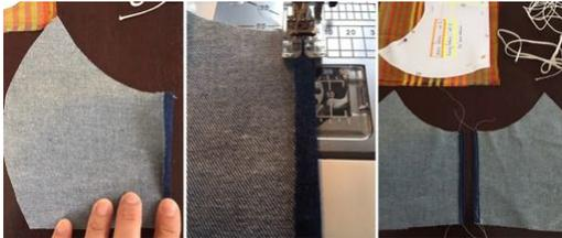
2...Sew center front seam. With right sides together, sew/serge center front seam of lining. Clip curve to ease. Repeat with the main fabric center front seam.
